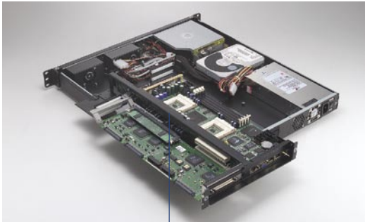
Butterfly backplane design supports two full-length 64-bit PCI expansion cards
