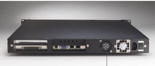
Rear 10-CFM cooling fan
