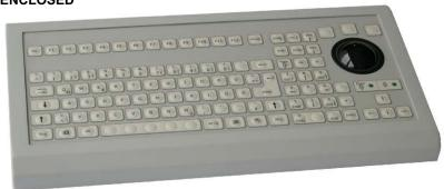
The keyboard and trackball are combined in one **compact**, robust steel enclosure. The unit has been designed to be used as desktop model.
