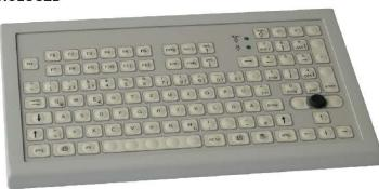
The keyboard and TouchStyk are combined in one **compact**, robust steel enclosure and will fit into 19" rack drawers (1HU) or can be used as desktop model.
